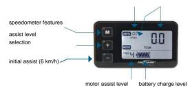
When the system is switched on by turning on the battery, the assist level is automatically set to 2. Using the "+" and "-" keys, the motor assist level can be changed from zero (no assistance) or from 1 to the maximum of 6.
